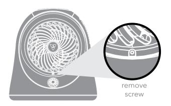
**3.** Twist Grill counterclockwise to unlock and pull out.
