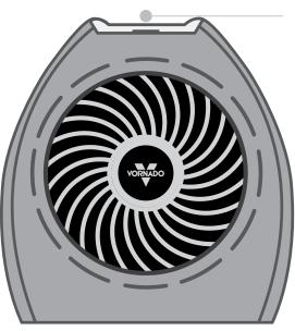
4. Press Power button & and select a Mode **(1)** Next, set thermostat to desired temperature using -/+. The SET TEMP and ROOM TEMP numbers will appear on the LCD Display. You may also select Fan Only by pressing **(1)**.
