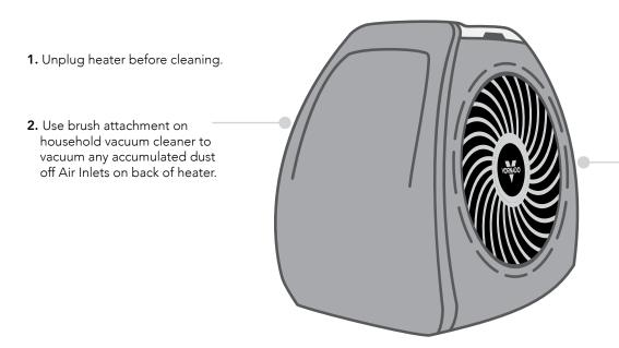
You should periodically blow out the heater with pressurized air to keep heat element and motor clear of dust, hair and debris that can build up inside the heater as it moves air during use. This also eliminates unwanted odors caused by accumulation of these particles inside the unit.
